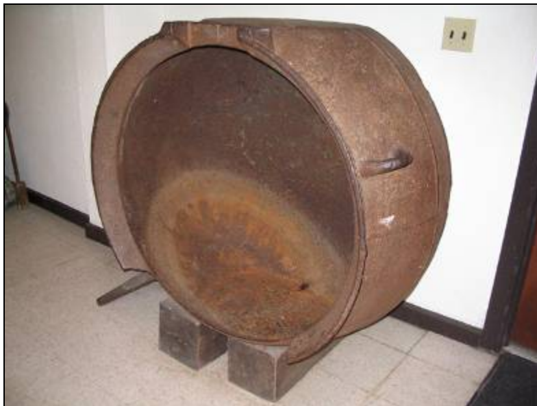
An 1865 iron try pot, once used by whalers to render oil from blubber. This one was recovered from Swains Island. (NOAA ONMS)
